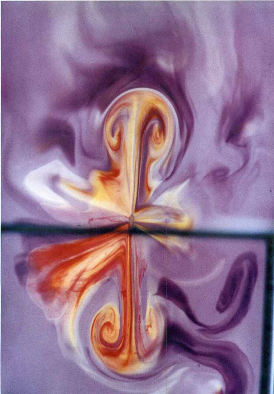
FIGURE 4. A dyed silicone drop of radius 2 cm rising through water rotating at 56 r.p.m. The aspherical prolate distortion is associated with the small air bubbles, visible at the nose of the drop, which generally accompanied the injection of the tracer particles (see figure 2 also).
